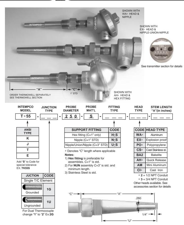
Thermowells protect probes from effects of fluid flow and pressure. These assemblies have a spring-loaded probes for positive contact against the bottom of the thermowell, as shown on cross-section diagram. Pressure and temperature ratings depend on the construction of the thermowell. See the thermowell section for more details.
