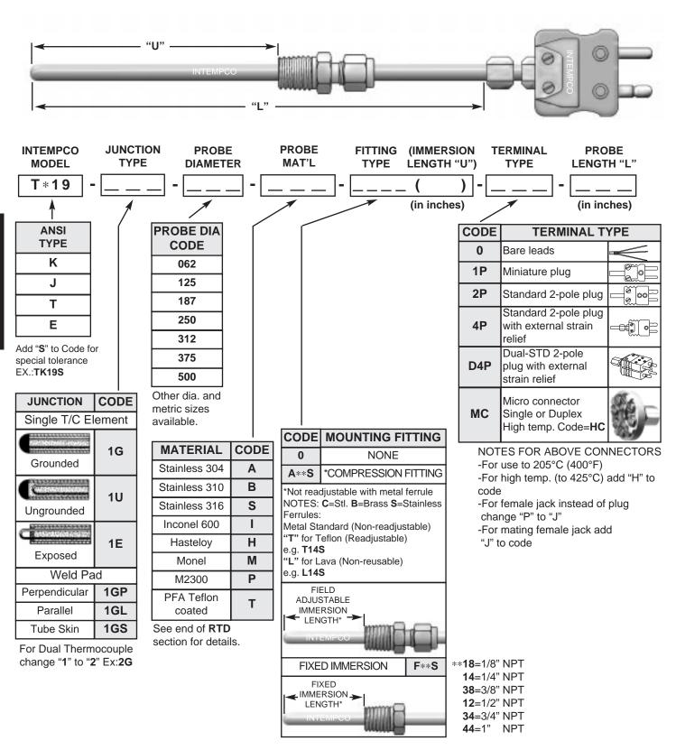
A general purpose probe made with various size prong connectors. These probes are very popular for educational and laboratory applications. INTEMPCO R\*19 probes are available with teflon coating. Teflon coated probes do not accept metalic compression fittings.
