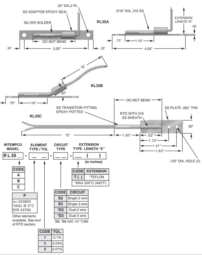
INTEMPCO **RL35** series surface temperature resistance element is designed to be cemented, clamped or bolted to a surface for temperature measurement. A specially designed moisture seal permits operation in extremely adverse conditions such as may be encountered on cooling equipment and cold water pipes. Teflon insulation and high temperature epoxy permit use at temperatures as high as 200°C (400°F).
