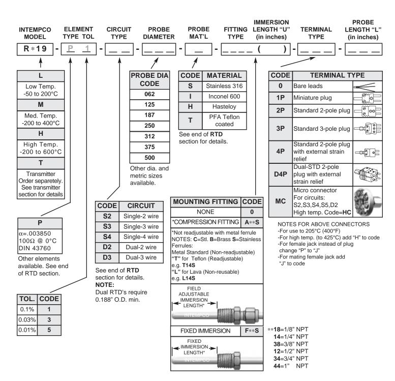
A general purpose probe made with various size prong connectors. These probes are very popular for educational and laboratory applications. INTEMPCO R\*19 probes are available with teflon coating. Teflon coated probes do not accept metalic compression fittings.
