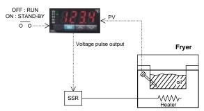
Control RUN/Stand-by selectable through external digital input
