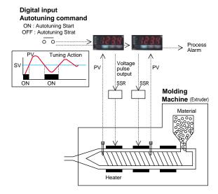
Auto-Tuning can be started/stopped through external digital input
