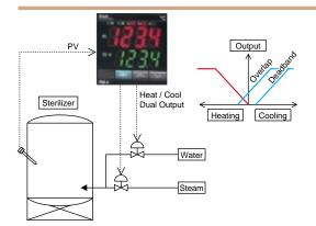
Cooling output and Heating output can be overlapped or a "Dead-band" set between them.
