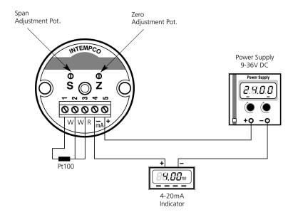
The diagram above represents the connection method to provide the 4-20mA with a current loop output. In most cases, the RT810 would take the form of a 3 wire output probe assembly. The output loop, the indicator and the transmitter are powered by a 9 to 36 VDC power supply. The indicator could be replaced by a controller, a data logger, etc.
