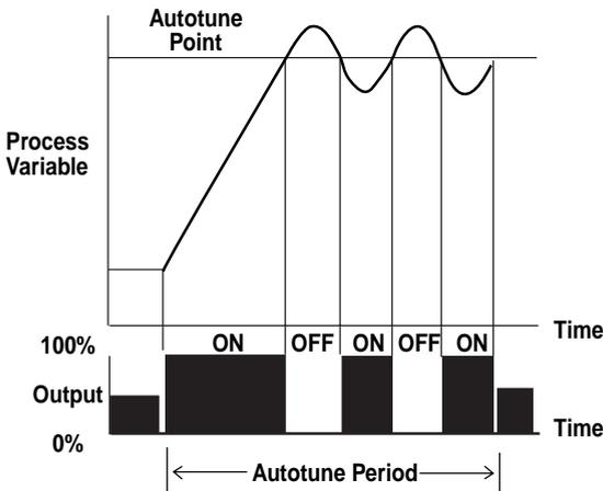
The PXZ then reads the reaction of these test signals on the process. Keep in mind that every process is different and therefore every reaction to the test signals is different. This is why PID parameters are not the same for different processes. The amplitude (L) or lag time which is the overshoot and undershoot of the system when autotuning and the time constant (T) which is the time the process takes to go through one On/Off cycle is measured. See diagram below.
