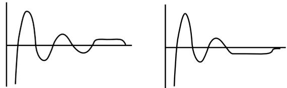
Integral action eliminates offset by adding to or subtracting from the output of the proportional action alone. This increase or decrease in output corrects for offset error within the proportional band in establishing steady-state performance at setpoint. It is not intended to correct for process disturbances. See the following diagram.
