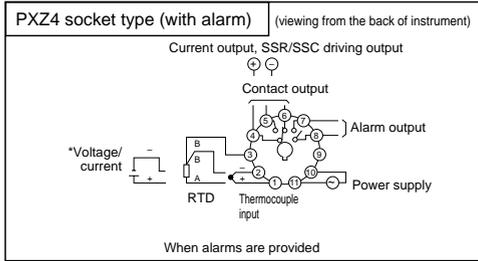
\* For current input, install the 250Ω precision resistor (accessory) before using the unit.
