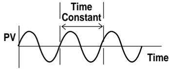
4. Widen the Proportional Band until only slightly unstable. This is the Proportional Band's Ultimate Sensitivity. The Proportional Band's Ultimate Sensitivity width will be defined as "P" when calculating the actual Proportional Band.
