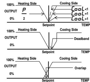
**bAL Balance:** Balance is used to pre-position the proportional band with respect to setpoint. With Balance (MV Offset) set at 50% the proportional band will be centered around setpoint. To move the band left or right, decrease or increase the balance setting respectively. Setting range: 0-100%
