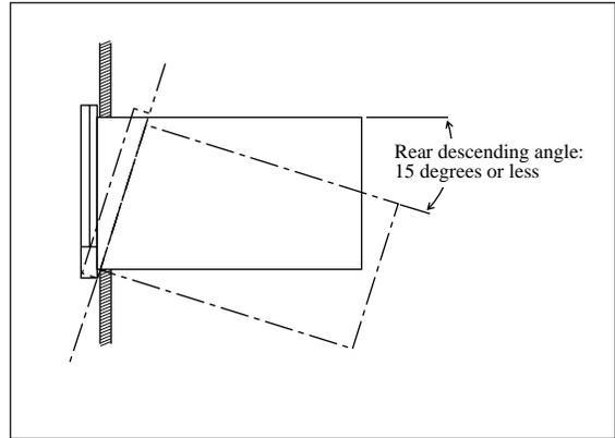
Figure 5-2 Installation angle
