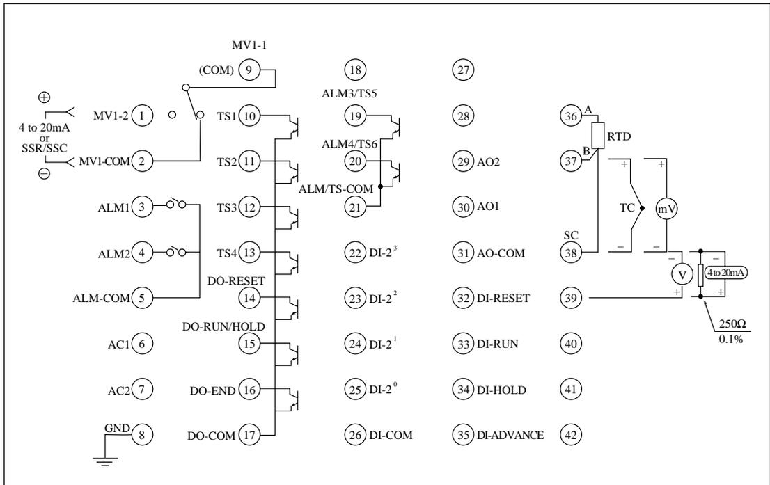
Figure 5-3 External Wiring Diagram
