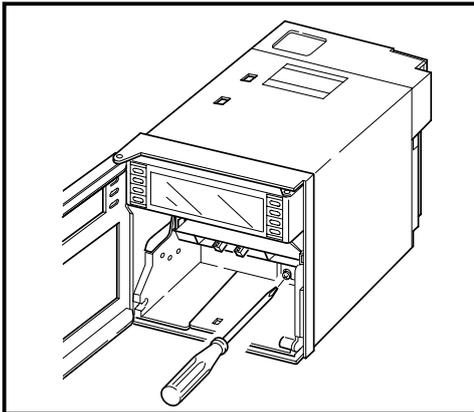
Loosen (counterclockwise turn) the lock screw and remove the unit.
