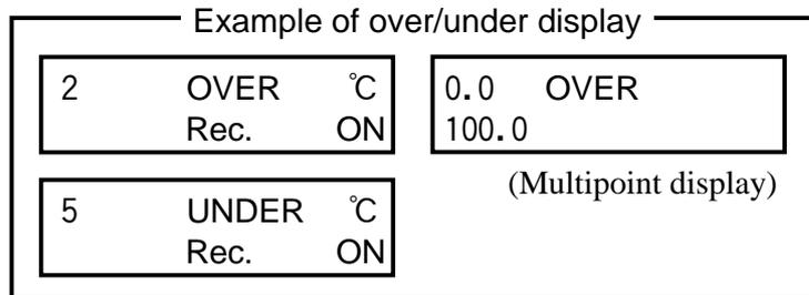
When voltage input is applied and the input signal cable breaks down or an over/under voltage is inputted, it is displayed as an abnormal input.
