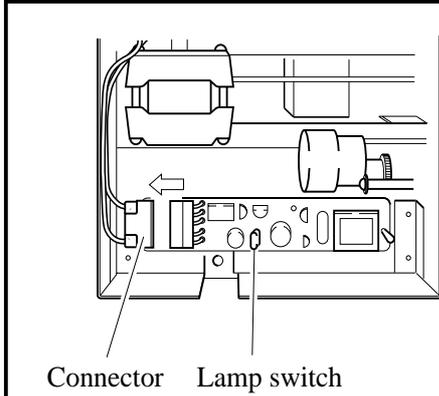
Remove the connectors(2 places) connecting the display unit to the main unit.
