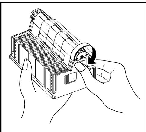
Shift the chart paper forward by turning clockwise the gear of the roller unit with hand.
