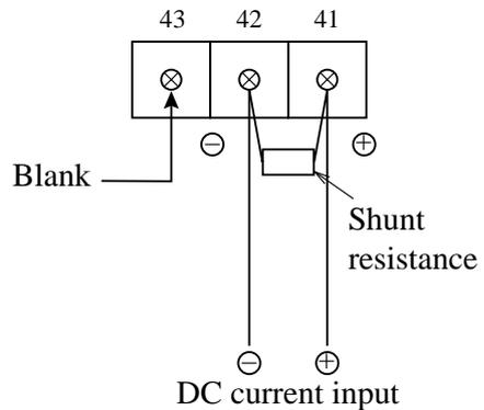
Example :  $10\Omega \pm 0.1\%$  shunt resistance is used for 4 to 20mA and 10 to 50mA input.
