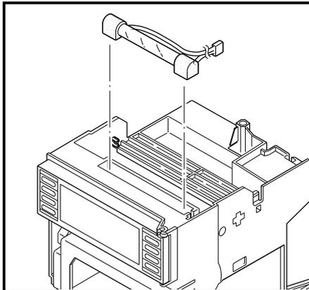
Remove the fluorescent lamp from the rear of the display unit.
