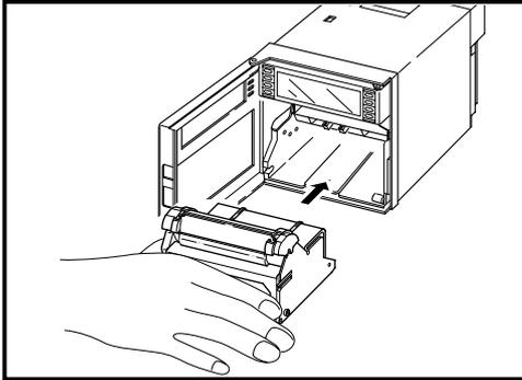
· Set the paper feed unit in its original position.
