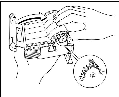
Insert the sprocket correctly in the perforations of chart paper. Move down the chart paper retainer (B) and set the paper on the roller unit.
