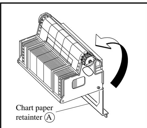
Transfer the chart paper which has been shifted forward, into the storage of the paper feed unit. Then set the chart paper retainer (A).
