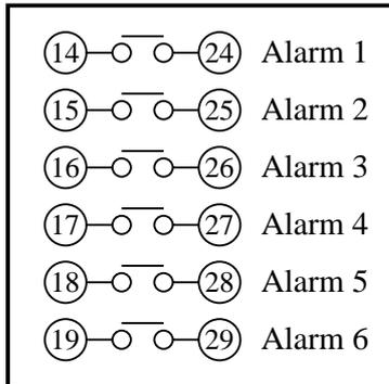
Note : If lamps are used on the outside, insert a resistor to prevent surge current.
