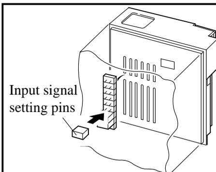
Change the setting of each channel pin on the printed circuit board in the unit.
