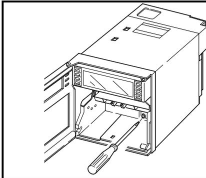
Loosen the lock screw (M4) in the unit with a Phillips driver.
