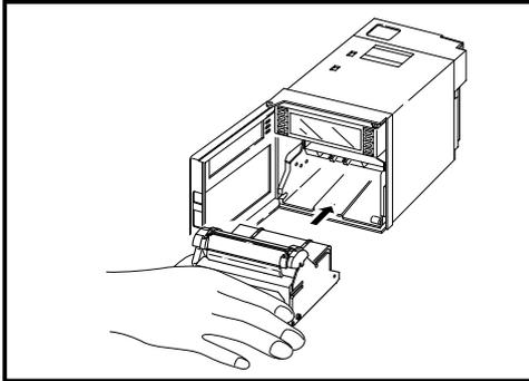
Mount the paper feed unit in the recorder. At this time, check that it is properly locked in position.
