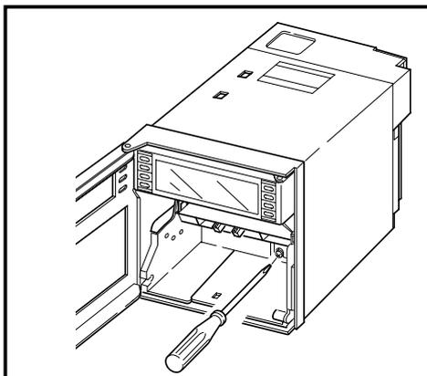
Loosen lock screw (M4), by using a (+) driver.
