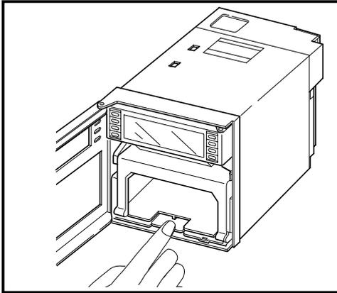
Open the front door and press down the paper feed unit drawout lever.
