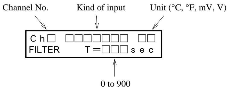
Note: When the kind of input is set to skip, indication, recording and alarm operations are not performed.
