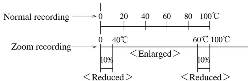
Note 1: Do not set the normal recording 0% value at the 100% recording position or the normal recording 100% value at the 0% recording position.
