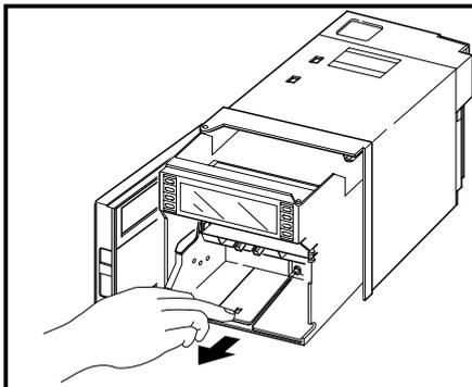
Hold the side or bottom of the frame and pull the unit forcibly to remove it from the case. It can be removed easily when the door is opened by about 90°.
