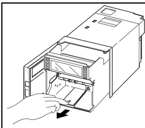
Hold the side or bottom of the main unit and pull it forcibly until it is removed.
