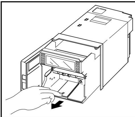
Remove the display unit from the main unit.
