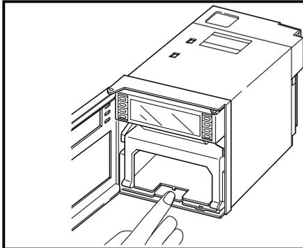
Open the front door and press down the paper feed unit drawout lever.
